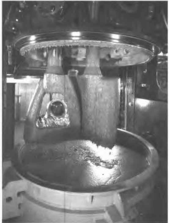
Mixing SRM propellant at Thiokol near Brigham City, Utah, in 1980.
