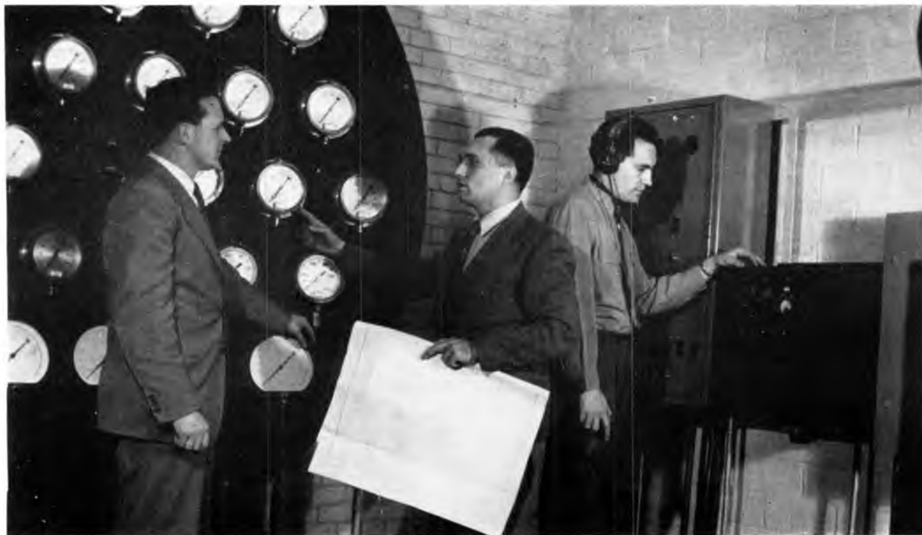
Dr. W. Sieber (Left) and Ernest Seiler, Scientists, along with I. G. Gaol, Electronics Engineer, checking the intricate instrument panel used in recording the reaction of a model guided missile under various amounts of pressure.
