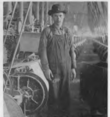
This photograph of John Garner was taken about 1916. Over the loom at left can be seen one of the early "filling boxes". Weavers filled their aprons from these boxes and carried the filling along to place in batteries where needed.
