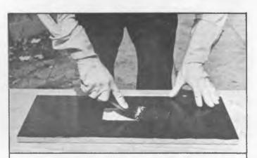
Remover is allowed to soak in until a wide-bladed putty knife can scrape off all paint layers in a continuous ribbon. If necessary, more remover is applied until scraper can cut through to clean wood.
