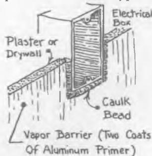
have shown that there is enough moisture loss through the perimeter of an outlet box to form a large ball of frost on the back face during extended cold periods. When this frost melts as the weather warms up, the water released can damage exterior paint films and promote rot inside the wall. In cold climates, sealing of the outlet boxes in insulated walls is especially important in rooms that generate a lot of water vapor, such as the bath and kitchen.
