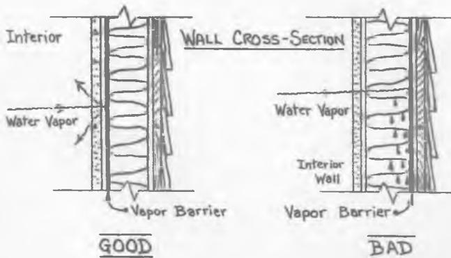
VAPOR BARRIERS are used to prevent moisture from getting inside the partitions in the first place. Vapor barriers should always be placed on the warm side of the insulation—NEVER on the cold side. For example, if you are pouring insulation in the attic floor, lay down a vapor barrier first. (Thin plastic sheeting is adequate.) With blanket insulations, be certain to place the kraft paper or aluminum-foil side toward the inside of the house.
