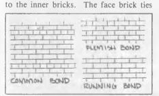
consist of occasional courses of eight-inch square bricks which present a normal-sized face but which extend eight inches back into the inner bricks. The Clay building has this feature, with the usual common bond on the side and rear walls, which has an unattractive header-course about every seven courses. Brick walls of
