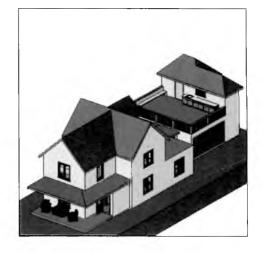
Architectural layout of the current structure, including post-1925 rear first floor reconstruction and later garage and apartment additions.
