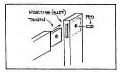
use of mortises and tenons necessitated prefabrication of the members on the ground, so the connections were given matching Roman numerals on the corresponding members for orderly erection. The Roman numerals were used because they are easily made with a chisel. These framing details involving the smaller framing members can be seen in the Constitution Hall Park outbuildings, which are all of a small size.
