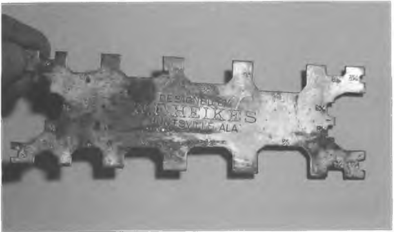
The device designed by William F. Heikes to measure the caliper of fruit trees and seedlings
